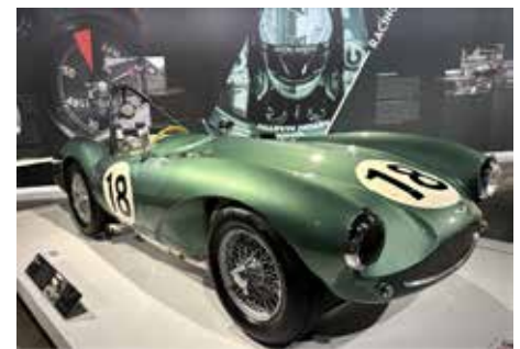
The DB3S's 2.9L inline-6 produced 217 hp and made possible a 150-mph top speed
